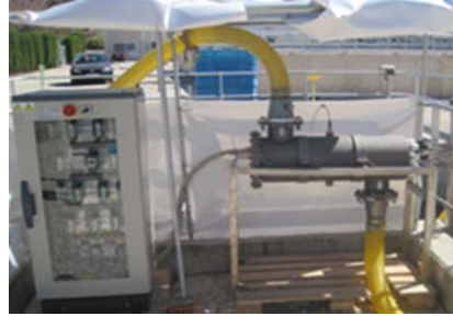
Photocatalysis UV in reactor of titanium dioxide
